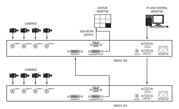
Figure 3. Connecting Multiple PMVC4s
